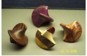
These are called "femispheres". A femisphere is turned from a block of wood that is first split in two along the center and then re-attached with double-stick tape, a paper joint, or a few drops of CA glue. It's turned between centers, then re-separated, one side rotated 90 degrees, and glued permanently together. Then the edges are sanded flush, which I will keep to a minimum for demonstration purposes.
