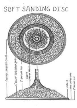
I use thin cheap double-sided carpet tape applied all across the leather to hold the sandpaper. Do not try to trim the carpet tape to the edge of the leatherinstead, just whack it off and fold the excess over onto the pad. The tape is so thin it will not affect the sanding at all. Then plop the pad down onto the backside of your sandpaper. I use 'A' weight, open coat, sterate coated alum. oxide sandpaper. Then trim the paper flush with the edge of the leather with a utility knife.
