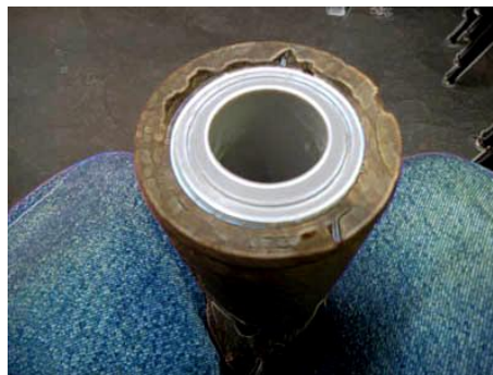
Grooves for inlaid filler
