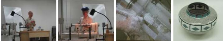
Andy glued the Corian, mounted the block and rounded the block and hollowed it out, a bit. The surprise is that Corian, that looks so much like a rock, being an acrylic resin, ends up giving fine, long shavings off of the tool. (See below.) Corian is not finished by a coating. A beautiful luster is achieved by sanding and then buffing with fine abrasives. Andy also mentioned that <u>very</u> hard tools
