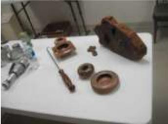
Kirk uses big pieces for big voids, powder for small voids. If he happens to have a mesquite piece with not voids, he cuts a groove – for instance, a groove around the top opening of a bowl. Kirk advised to avoid putting inlays inside, they are hard to sand down.
