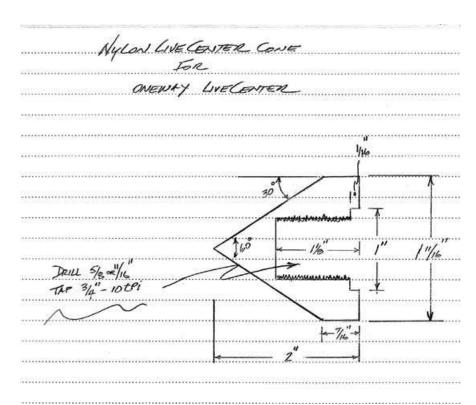
This makes a nice cone center, but other shapes can be made with the same general technique and the excess Nylon from the blank. Special Jam chucks come to mind, but at least this gives one a start. (It also fits the Jet 16/42 live center Darrell). Mind the loads and loads of excess stringy plastic, but this thing works just fine with regular tools doing the cutting.
