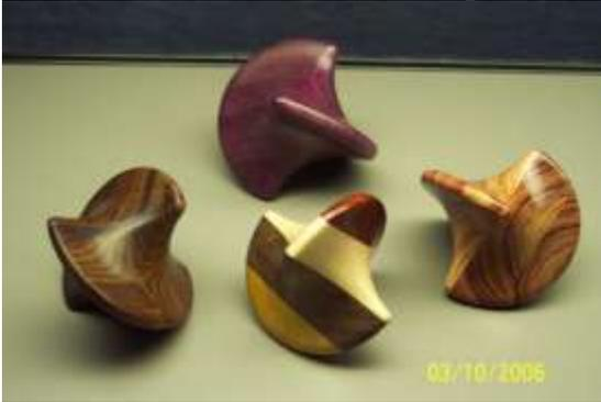
These are called "femispheres". A femisphere is turned from a block of wood that is first split in two along the center and then re-attached with double-stick tape, a paper joint, or a few drops of CA glue. It's turned between centers, then re-separated, one side rotated 90 degrees, and glued permanently together. Then the edges are sanded flush, which I will keep to a minimum for demonstration purposes.
