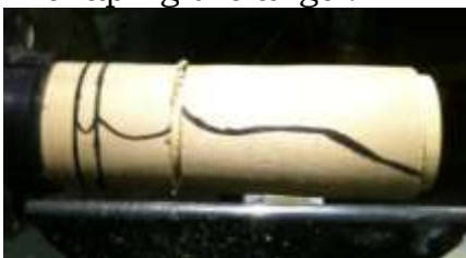
rounded blank, with roughed out plan (halo, head, body)
