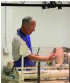
He likes bowl gouges and thinks a lot of work should be done with them. He grinds his tools at a 60 grit wheel, because the edge can be made quite sharp and, under magnification, reveals a finely toothed edge that aids in making slicing cuts. He talked about using more moderate grades of high speed steel because of the cost
