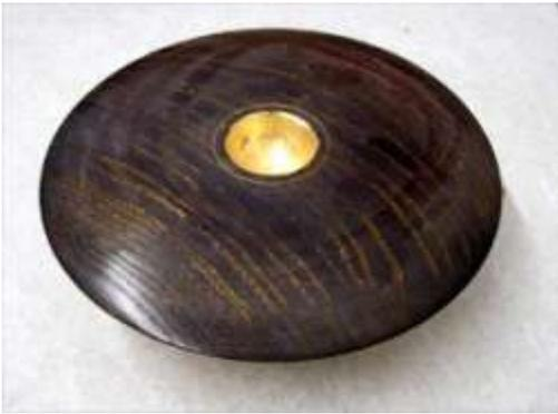
He focused on making insets for expansion jaws and their opposites, tenons, measured to fit the chuck jaws at their closest to being round, for maximum hold on the wood. He pointed out that in expansion mode a good amount of wood needs to remain, surrounding the inset to make sure the outward pressure doesn't split the blank.
