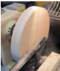
8. In the center of the platter, make a dovetail tenon of suitable size for your 4 jaw chuck (a tiny bit bigger than the closed chuck, use calipers to check.) Keith Gotschall says 1/8 to 3/16 deep is good enough. To start, choose the larger. The dovetail will give you added safety, but don't get too cocky or clumsy with the tools. Don't bother with cleaning up the tenon or decoration because you will turn this tenon away later.
