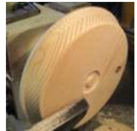
10. Take the bowl off of the screw chuck and reverse the platter to hold it in the expansion jaws. Check that the jaws are tight and seated firmly against the bottom of the tenon.
