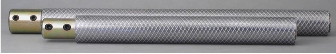
Figure 7 – Finished Removable Tool Handle
