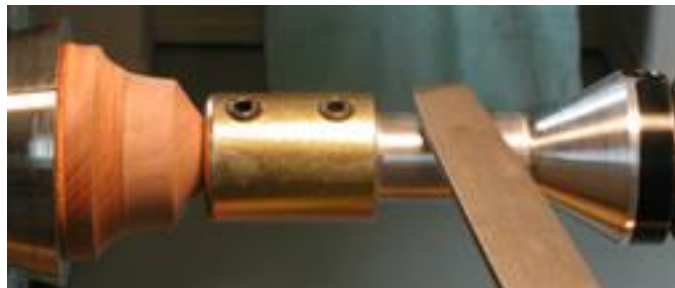
Figure 3 – Filing the Insert to Fit the Tubing
