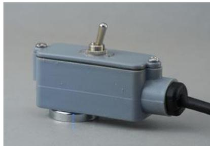
Figure 13 – Shop Made Remote On/Off Switch
