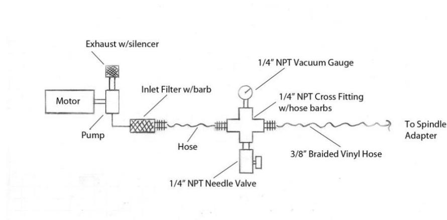
Figure 9 – Schematic of a Typical Vacuum System
