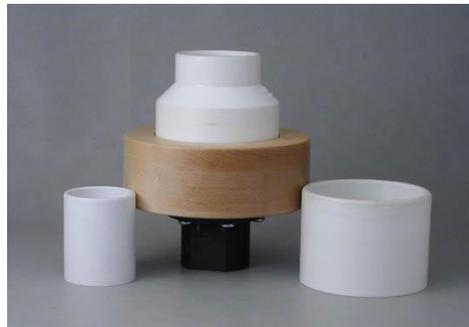
Figure 11 – Shop Made Vacuum Chucks
