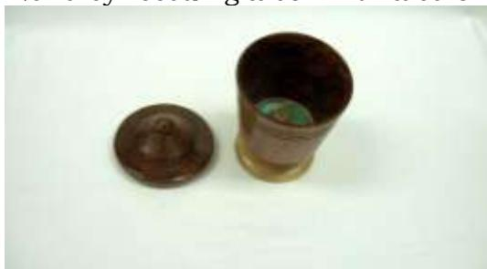
Special consideration must be given to the method of attachment of any added feature, consider the size of the hole and any tenon necessary. It was pointed out that it is better to have a bevel instead of a straight edge on the two pieces to be joined to insure a better fit and less obvious glue joint. Make the tenon proud so that you have something to work with. Now is the
