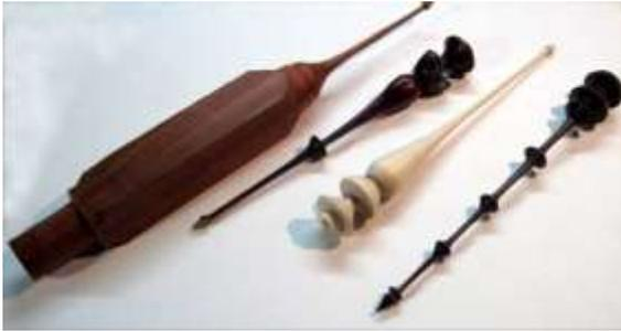
Start at the distal end of the finial and work back toward the chuck in 2 to 3 inch increments, leaving the untouched area as support. With each section turn the work down, refine shapes, sand it down (rough) and finish sanding (fine). Don't go back to this section unless you are willing to take the consequences.
