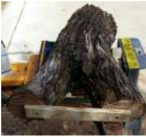
crotch vase with long leaves. He first took the group from choosing the log to preparation. It was noted that, where the two branches ended, he bridged the two branches with a length of plywood (3/4 inch?) screwed into the ends of the wood. This would allow the whole log to be turned between centers to prepare it for a glue block at the base, attached to a screw plate. Once the piece had been firmly attached to the plate and the plate attached to the headstock, the
