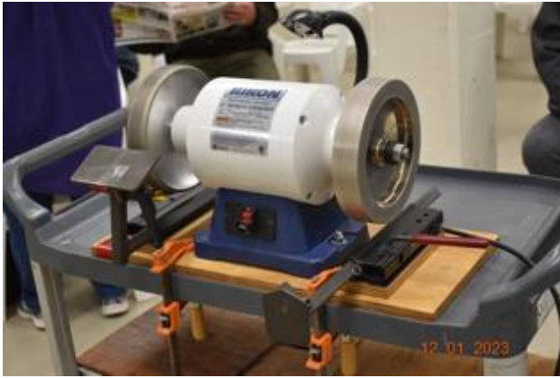
Grinder set up - 2 CBN wheels and Wolverine jig
