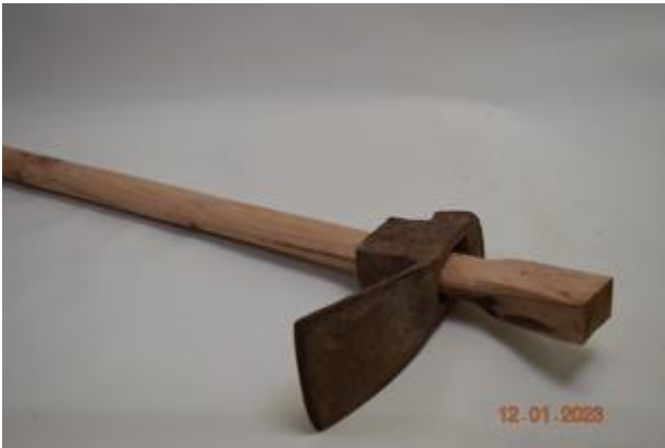
Tom Canfield Tapered head, offset turned handle for antique Adz Red Oak
