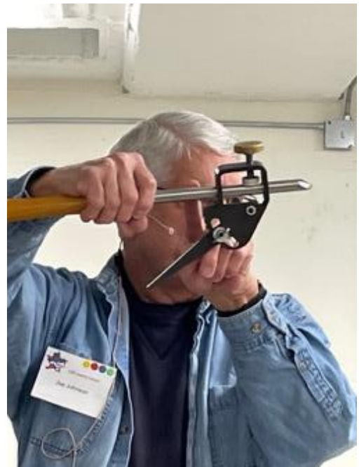
Showing the 2" gouge protrusion
