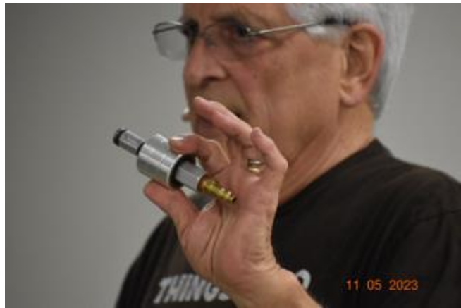
Adaptor to connect vacuum pump to lathe headstock and vacuum chuck
