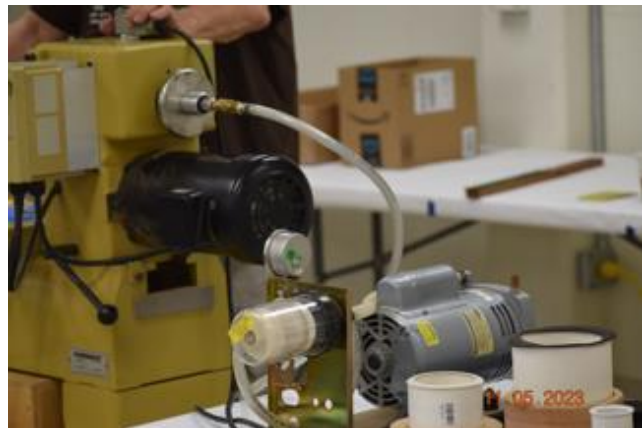
Complete set up with rotary vane vacuum pump and vacuum adaptor
