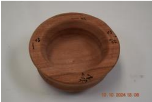
Tom Canfield, Red Iron Bark. Shows warpage and shrinkage from green turned wood
