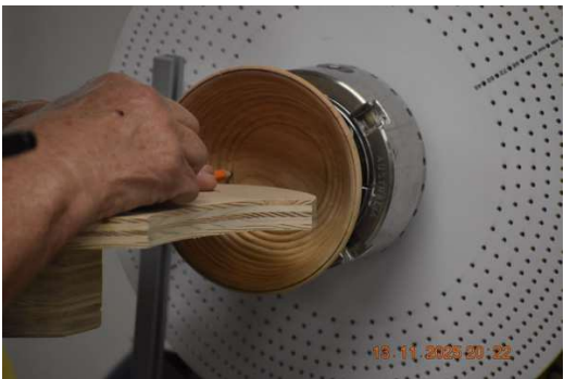
Marking using pencil platform
