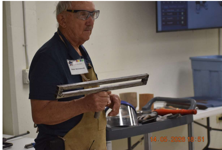
Dale showing the trap/backrest which holds the D-Bar/boring tool
