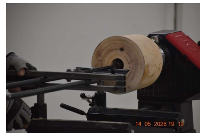
Trap with D-bar/ boring bar/hollowing tool in position
