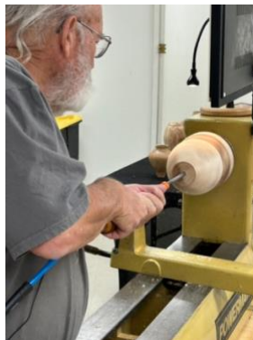
Drilling w/ air assisted Gun Drill
