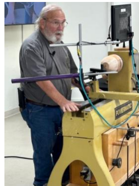
Prepping Hollowing system
