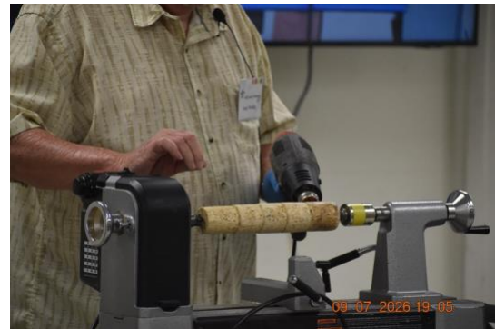
Speed up drying with heat gun
