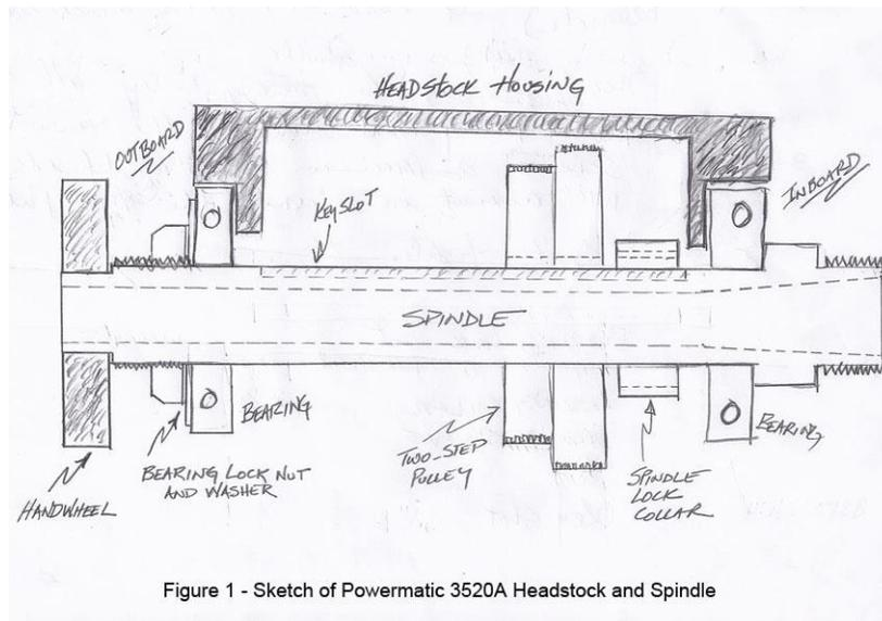
Figure 1 - Sketch of Powermatic 3520A Headstock and Spindle
