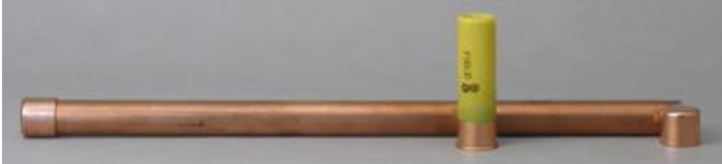
Figure 5 – Lead Shot Filled Copper Tube for Additional Weight
