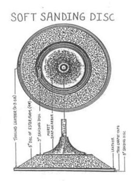
semi-circular scratches, but the floating action eliminates these scratches. Also, the softness of the foam and the tapered edge allows the pads to conform to concave surfaces with gouging.
